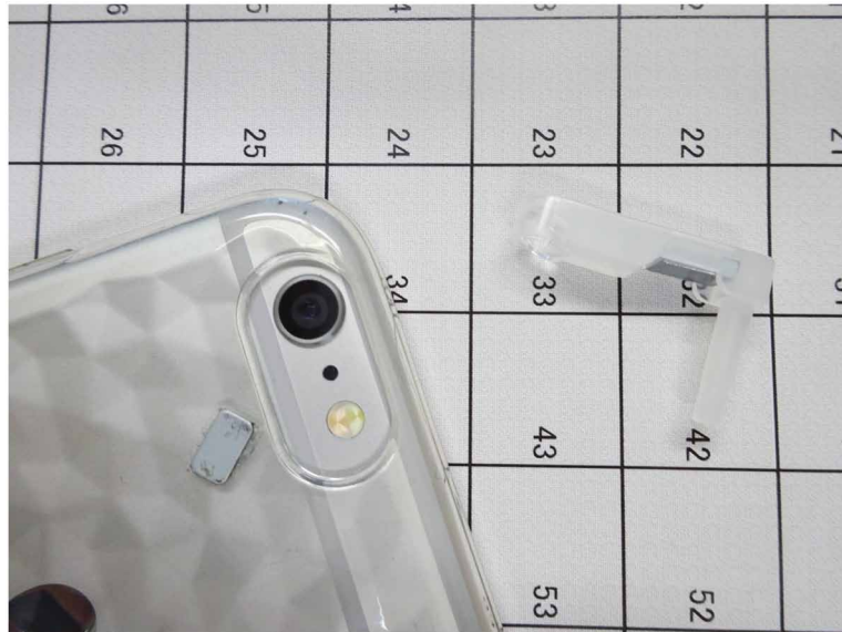
Figure 2. Handmade sheet generated by ScreenCode and a specially designed lens
