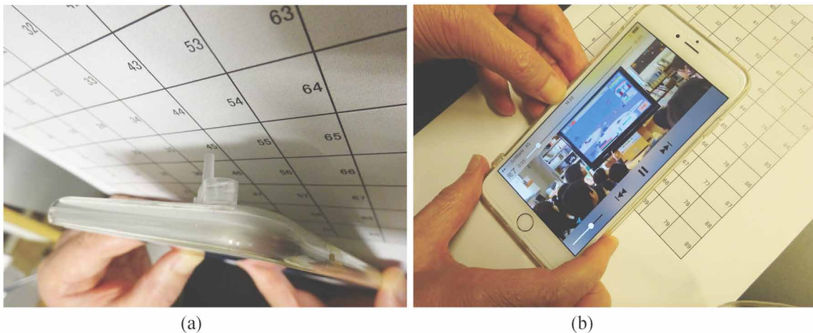
Figure 7. (a) Special lens attached to an iPhone and (b) snapshot of iPhone screen (school activity movie), focusing on ScreenCode dot codes
