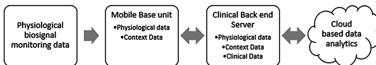
Figure 11. Structure of cloud based data analytics platform
