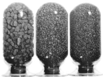
Figure 2.6: Alloy precursors for fixed-bed Raney catalysts.
