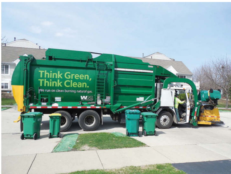
Figure 1.1: Garbage truck that utilizes natural gas.
