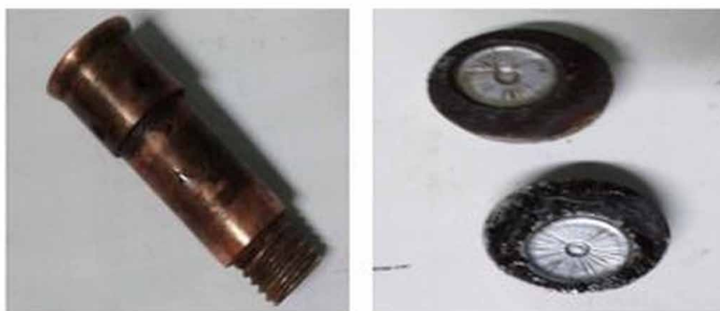
Figure 2. EN19 tool for ECM experimentation (Tiwari et al., 2016)
