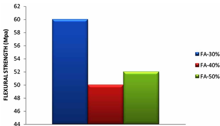
Figure 9. Flexural Strength of 30 wt%, 40 wt% and 50 wt% fly ash filled polyester composite
