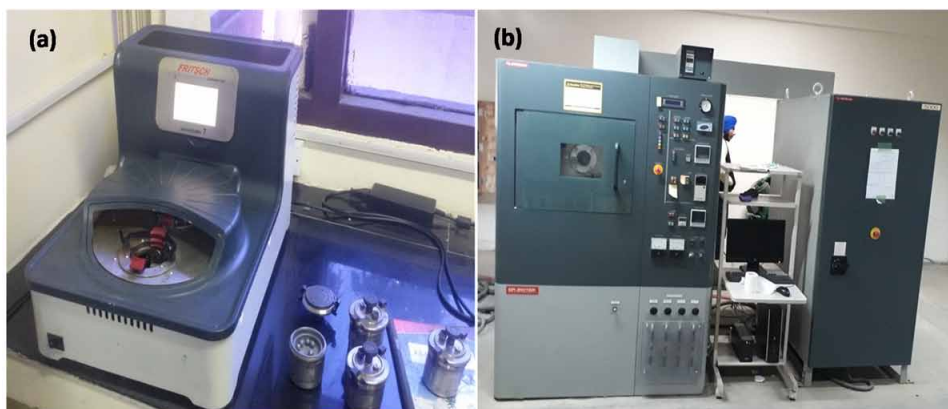
Figure 1. (a) High energy planetary ball mill and (b) spark plasma sintering (SPS) machine
