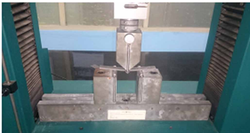
Figure 5. Flexural strength using three point bending test
