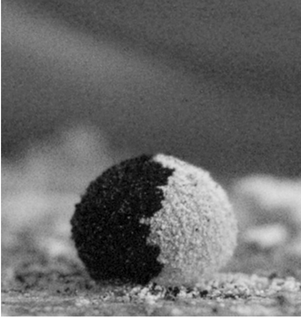
Fig. 9.5: Forty-microliter water Janus marble coated with carbon black and Teflon.
