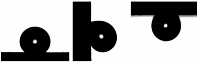
Fig. 6.9: A 10- \mu\text{l} droplet deposited on a surface built of lycopodium particles.
