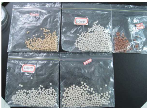
Figure 3.6: Comparison of five types of clay ceramsite and ceramsite with different fly ash sintered by muffle furnace: (a) 100% bentonite ceramsite, (b) 50% bentonite: 50% fly ash ceramsite, (c) clay ceramsite, (d) 75% bentonite: 25% fly ash ceramsite and (e) 25% bentonite: 75% fly ash ceramsite.
