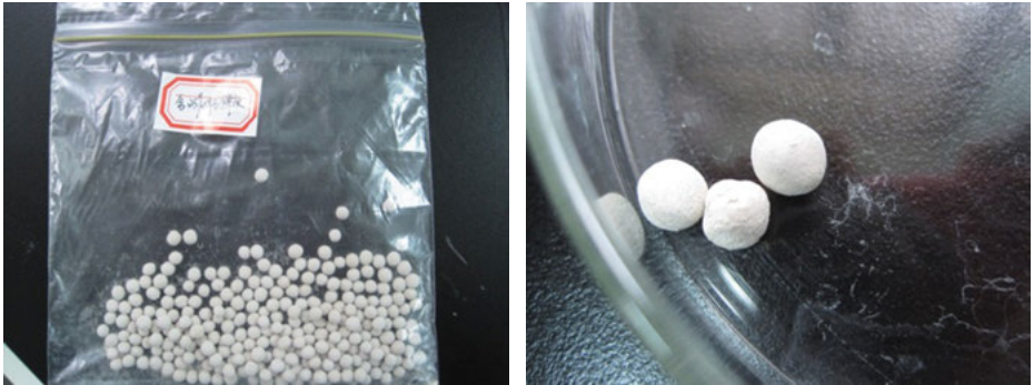
Figure 3.8: 75% bentonite: 25% fly ash ceramsite sintered in muffle furnace.
