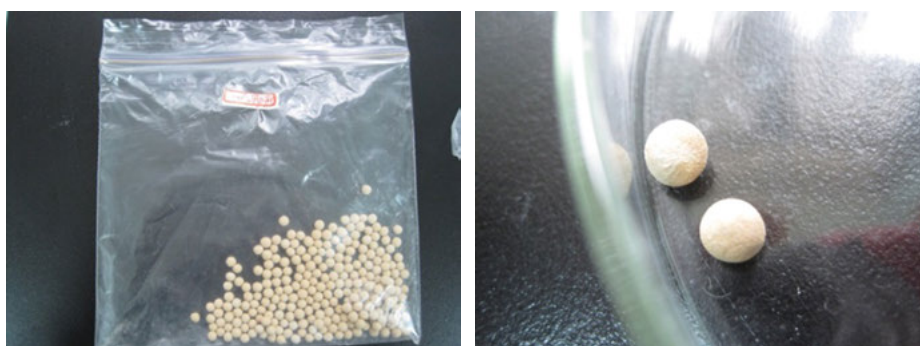
Figure 3.7: 100% bentonite ceramsite sintered in muffle furnace.
