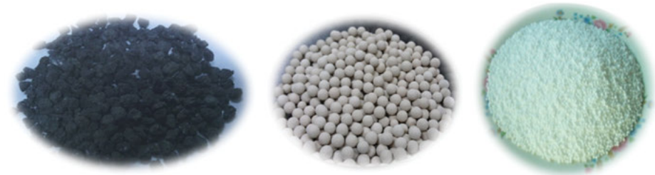
Figure 7.1: Volcanic rock, fly ash ceramsite and styrofoam filter beads.
