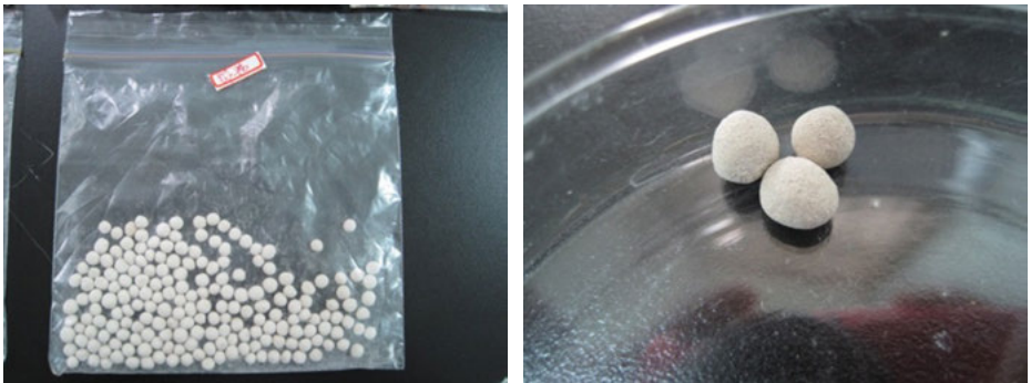
Figure 3.10: 25% bentonite: 75% fly ash ceramsite sintered in muffle furnace.
