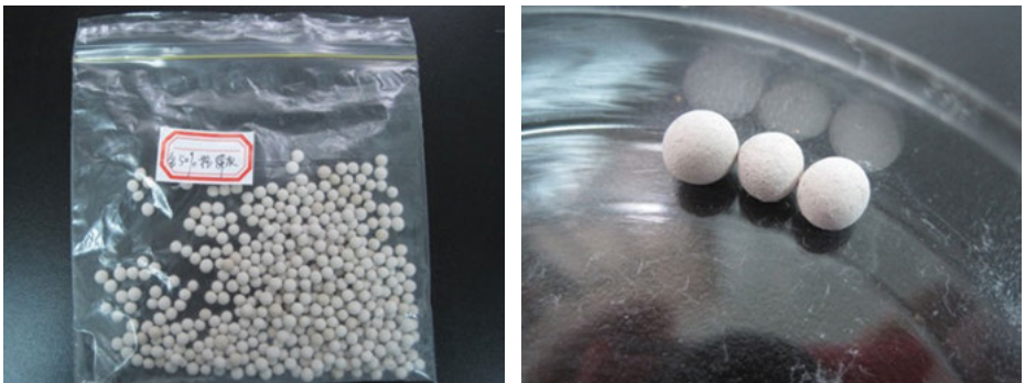
Figure 3.9: 50% bentonite: 50% fly ash ceramsite sintered in muffle furnace.
