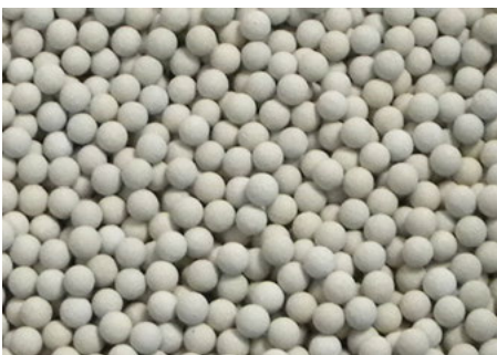
Figure 3.28: Fly ash ceramsite products of pilot sintering experiment.
