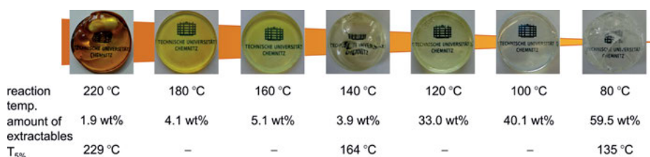
Fig. 5.21: Images of monolithic samples synthesized from BADGE and APSI with a molar ratio of 1:2 at different temperatures with their extractable content. T 5% = temperature at which 5% weight loss is recorded by thermogravimetric analysis at a heating rate of 10 K·min -1 under air. Reprinted and adapted from Ref. [71], Copyright 2017, with permission from Elsevier.
