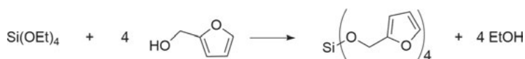
Scheme 2.2: Synthesis of the twin monomer tetrafurfuryloxysilane (TFOS) by transesterification of tetraethoxysilane (TEOS) with furfuryl alcohol under release of ethanol.
