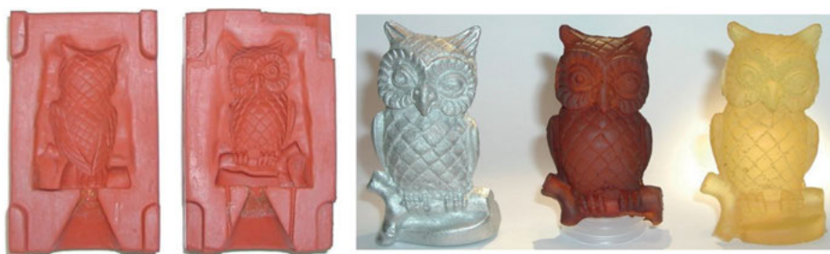
Fig. 4.2: Photographs of hybrid materials which show owl shapes (right) produced in a casting mold (left) by STP. The hybrid materials were obtained by lactic acid-catalyzed polymerization and annealing at 200 °C under argon (yellow owl) as well as 175 °C under air (red owl). For comparison, a cast tin owl (gray) is shown [28]. Reproduction with kind permission of Tina Mark.
