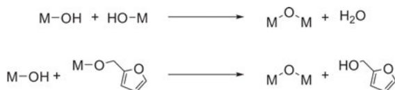
Scheme 3.9: Illustration of the condensation reactions providing metal oxide/metalloid oxide, water, and furan-2-ylmethanol. M denotes the central metal or metalloid atoms of the precursors.
