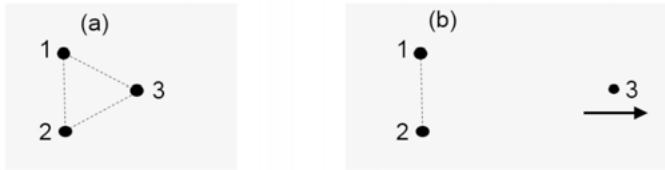
Figure 6.1: Cluster-separable interaction in a system of three particles. (a) Three particles interact at close distances. (b) When particle 3 is removed to infinity, its interaction with 1 + 2 vanishes, and the dynamics in 1 + 2 acquires a form characteristic of a two-particle system.
