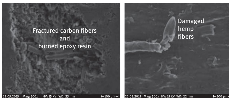
Figure 5.3: SEM micrographs showing fractured carbon fibers and hemp fibers in samples with 10.0 mm diameter hole drilled at f = 0.05 mm/rev and v = 20 m/min [17].
