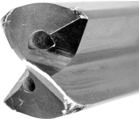
Figure 1.3: Showing that the maximum wear occurs in the vicinity of the drill corner.
