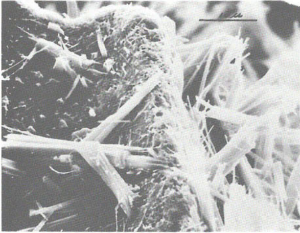
Figure 8. Scanning electron micrograph showing pitted glass fragment altered to acicular erionite in an ash bed from Jersey Valley, Nevada. (From Mumpton, 1973a.)
