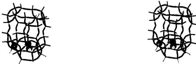
Figure 18b. A stereoscopic view of the framework of chabazite illustrating the main adsorption cavity or cage and the approximate location of the three cation sites. Site I in the center of the double 6-ring is at the origin of the unit cell and provides for a near octahedron of oxygen atoms. There is one site-I cation per unit cell. Site II is located near the center of the 6-ring but displaced away from site I into the main cavity. There are two site-II cations per unit cell. Site III occurs in 6 pairs of positions, each pair about 1 Å apart and near the tilted 4-ring. The locations indicated in the figure are approximate. (From Breck, 1974, Fig. 2.20.)
