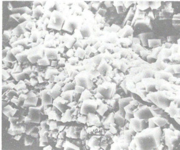
Figure 8. Scanning electron micrograph of chabazite rhombs from a lacustrine tuff along Beaver Divide, Wyoming. The crystals are several \mu\text{m} in diameter and commonly intergrown. (From Mumpton and Ormsby, 1976.)
