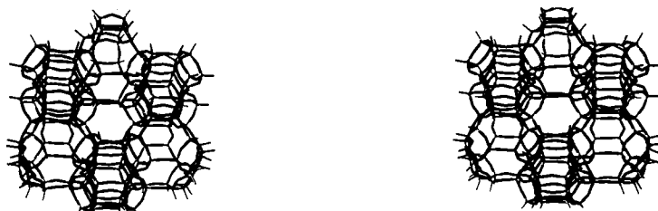
Figure 8. Stereoscopic view of the framework of erionite. The view is parallel to the c-axis and shows the stacking sequence of the 6-rings. The sequence is AAB. AAC. The framework consists of double 6-rings, D6R units, and S6R units which are arranged in parallel planes perpendicular to the hexagonal axis. Because of the stacking sequence, the c-dimension is 15 Å, i.e., 6 times the 2.5 Å spacing of a single 6-ring.
