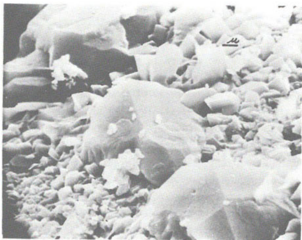
Figure 11. Scanning electron micrograph of large analcime crystals in a matrix of micrometer-sized crystals of potassium feldspar from a tuff near Barstow, California. (From Mumpton and Ormsby, 1976.)
