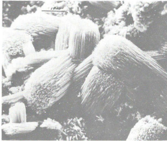
Figure 7. Scanning electron micrograph of erionite from a tuff near Hector, California. The bundles are about 20 \mu\text{m} long and about 10 \mu\text{m} wide and contain several hundred needles, each about 0.5 \mu\text{m} in diameter. (From Mumpton and Ormsby, 1976.)
