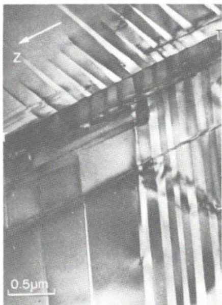
Figure 10. Nucleation of (\bar{1}01) hornblende lamellae at a (100) twin boundary T-T in grunerite. From Gittos et al. (1976).
