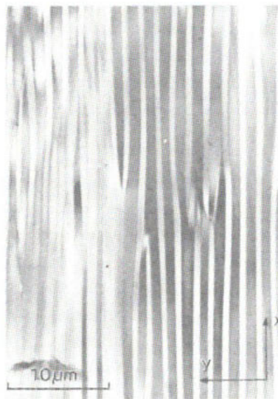
Figure 22 (above, left). Exsolution in anthophyllite. In localized areas the precipitates are isolated, "wavy" particles. Between them are smaller (010) platelets, some of which have nucleated on the (100) faults (shown by arrows).
