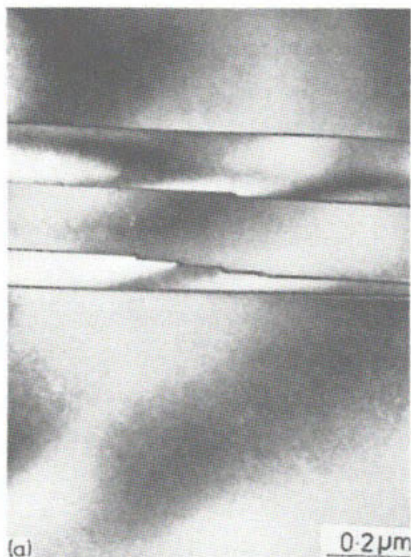
Figure 11. Grunerite lamellae in hornblende showing growth ledges. From Gittos et al. (1974).
