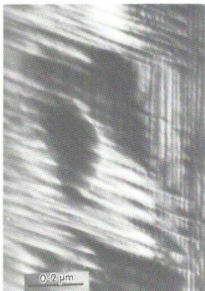
Figure 20 (above, left). Coexisting (\bar{1}01) and (100) exsolution lamellae in tiroditite. The (100) lamellae are vertical. (Phakey and Ghose, 1974, unpublished electron micrograph)
