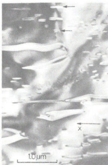
Figure 22 (above, left). Exsolution in anthophyllite. In localized areas the precipitates are isolated, "wavy" particles. Between them are smaller (010) platelets, some of which have nucleated on the (100) faults (shown by arrows).
