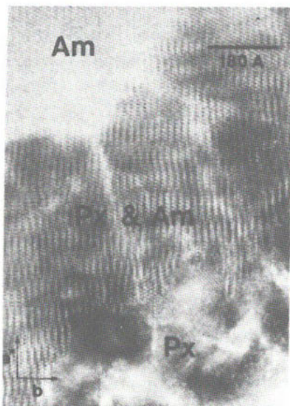
Figure 26 (to the left). Amphibole replacing pyroxene in a uraltite by a bulk mechanism along a reaction front; this is a crystallographically oriented reaction. The amphibole-pyroxene interface in this case is inclined to the viewing direction (the c -axis), resulting in moiré contrast where the two structures overlap. (After Veblen and Buseck, 1981.)
