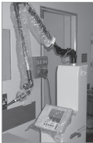
Figure 6.1: CO 2 laser comprising hand-held delivery device connected to generation chamber via a series of articulated arms and mirrors
