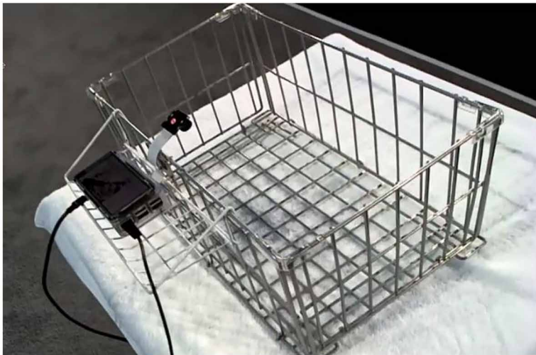
Figure 8. Shopping kart with IoT enabled raspberry pi and camera
