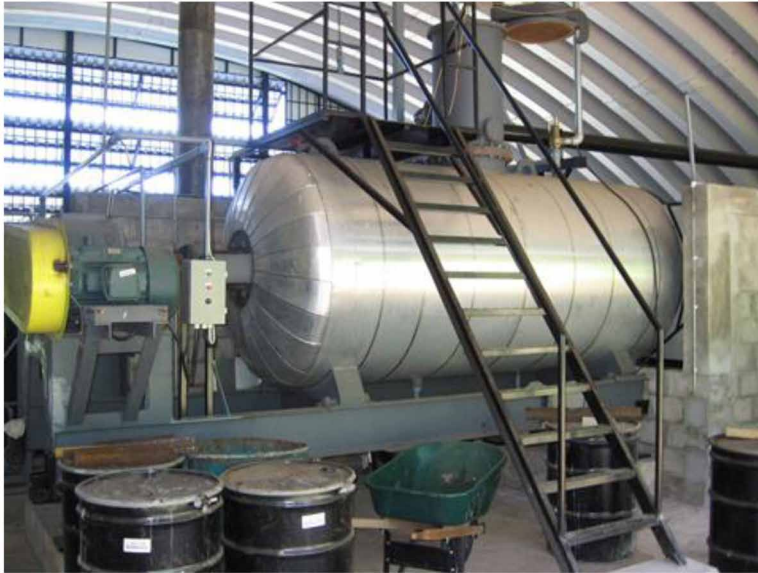
Figure 6. Harnessing of boiler discharge to steam cooker for rendering raw materials. Water vapor from the cooker is condensed and reused for crop irrigation.
