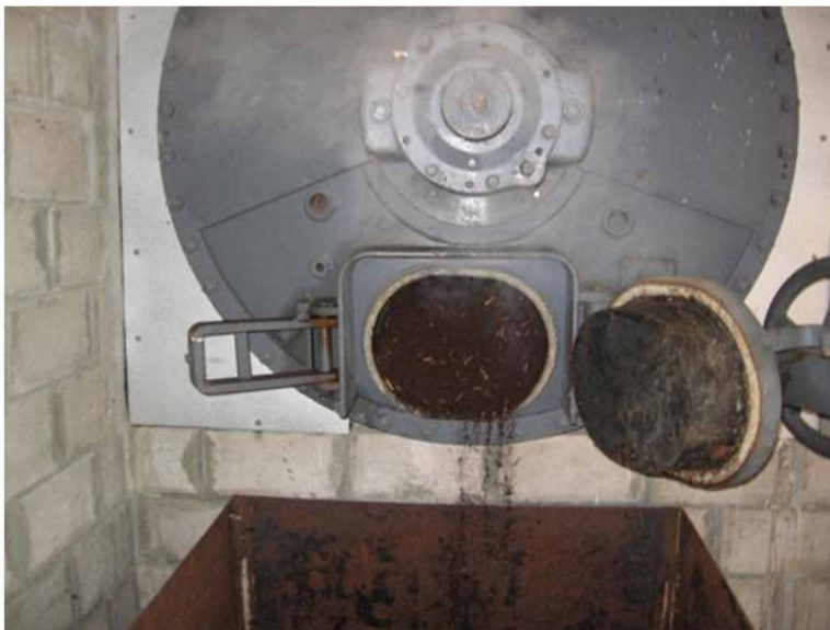
Figure 7. Discharge view from steam cooker and finished livestock feed protein supplement from cooker
