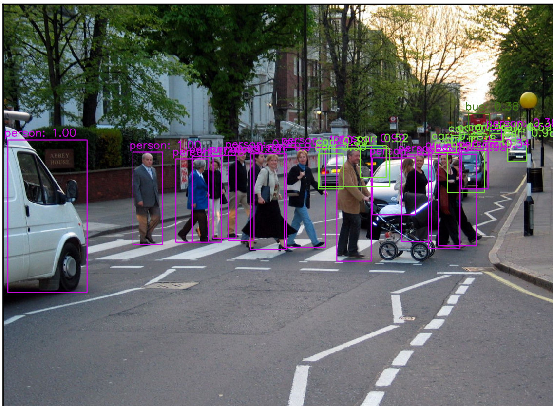
The output of an object detector. The vehicle on the left is wrongly classified as person, but the rest of the objects are classified correctly.
