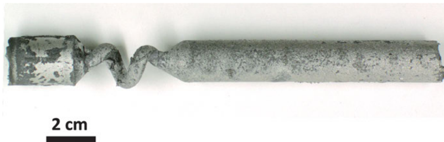
Figure 6: Equiatomic FeCoCrMnNi single crystal produced by investment Bridgman casting. Image courtesy by U. Glatzel, University of Bayreuth [52].
