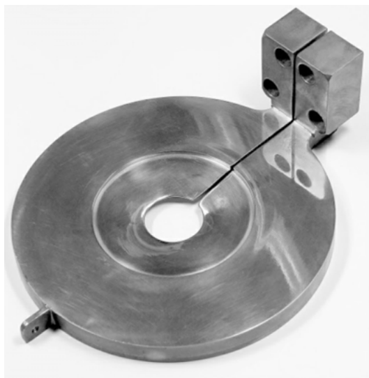
Figure 4: High-frequency one-turn inductor for FZ melting of conducting materials. Adopted from Ref. Lüdge A. et al. [6].
