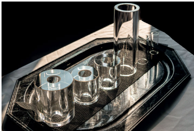
Figure 7: Transparent tubes forming the growth chamber of a mirror furnace. From left to right: single crystalline sapphire tubes for gas pressures up to 30 and 15 MPa, correspondingly; fused silica tubes for pressures up to 5, 2 and 1 MPa, correspondingly. Courtesy of Scientific Instruments Dresden GmbH (SciDre).
