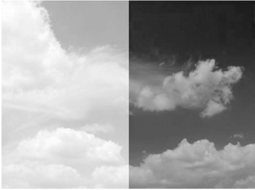
Figure 3.7: The visual effect with a polarizer improvement (from Internet). Left: the imaging was obtained without polarizer; Right: the imaging was obtained with polarizer.
