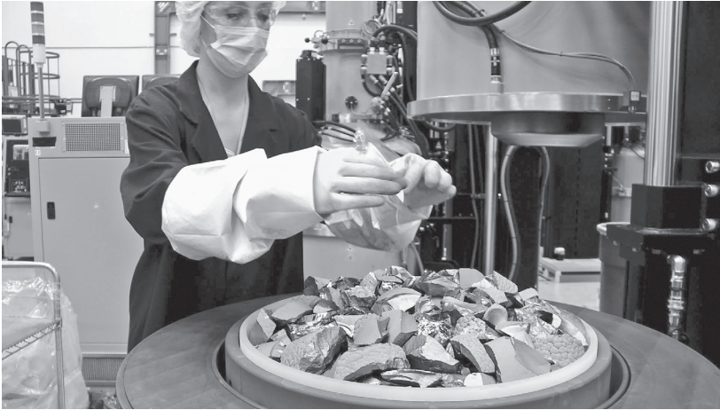
FIGURE 3. The Czochralski method for purifying silicon is still the basis for monocrystalline silicon photovoltaics today. (Photo: SolarWorld Industries Americas, Inc.)
