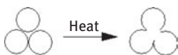
Figure 7.29: Schematic diagram of the sintering process. Typical pore sizes between 0.1 and 10 \mu\text{m} . Porosity 10–20% with polymer; 80% with metals.
