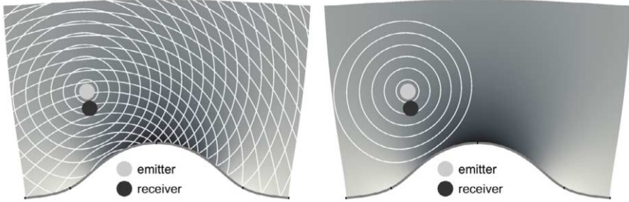
Fig. 2. – The renormalization: Subtract the direct interaction between adjacent points (right) from the full interaction (left). Only the scattered waves that probe the geometry remain.
