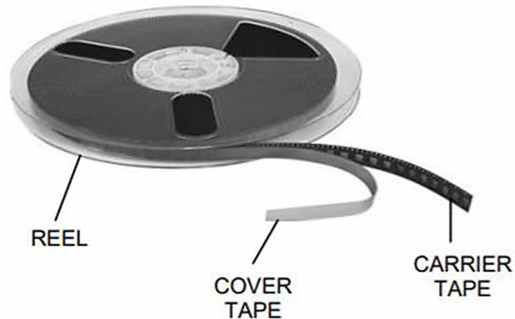
Figure 3. Kanban reels for SMD (Surface Mount Device) materials (Adapted from [Mini-Circuits, 2018])
