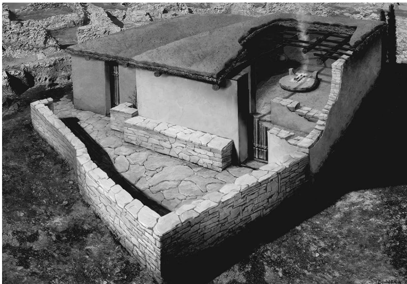
FIGURE 9.5. Illustration of the Central Megaron Complex showing wall construction technique, use of exterior wall plaster, and freestanding location. Also note the stone bench in the courtyard, which would have been used during social gatherings (drawn by K. Donner).
