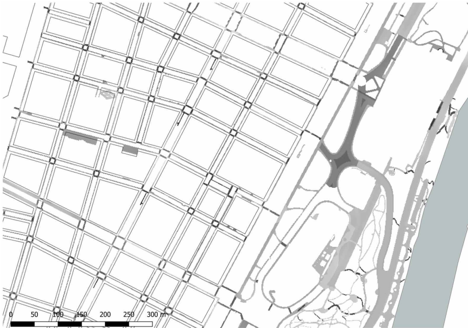
Figure 1. Neighborhood level: the cost raster. The color, from light gray to dark gray, represents increasing impedance, that is increasing “cost” of walking through the cell.
