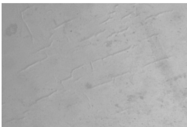
Figure 6.5: Cracking on a NR film.
