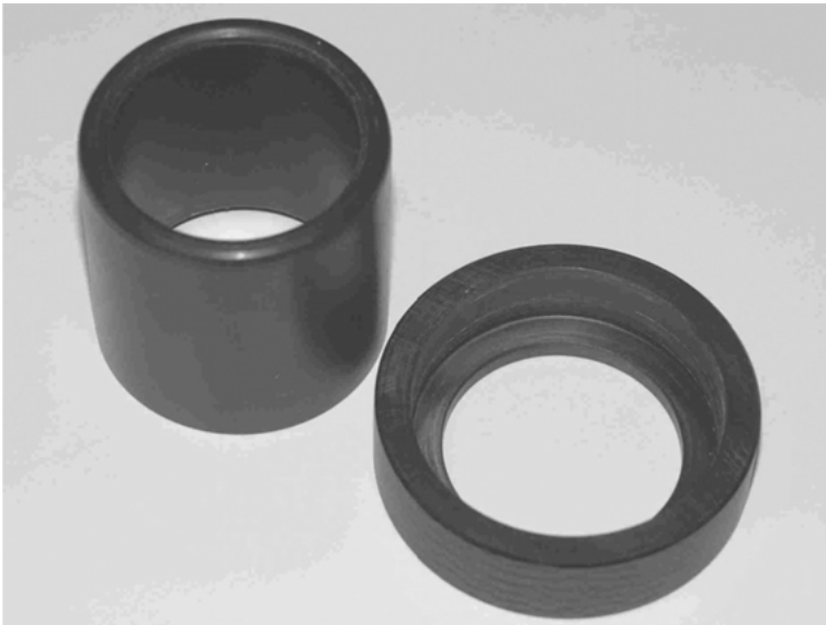
Figure 12.3: A simple sample holder can be made from a plastic tube. In this example, a cap to secure the sample can also be seen.
