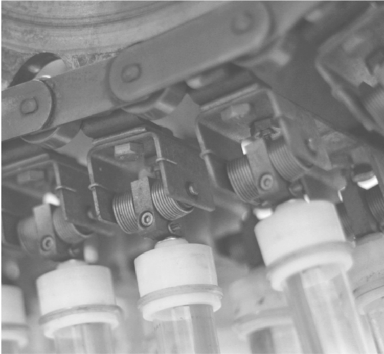
Figure 9.2: An example of the way in which condom formers can be attached through the spinner to the chain. Reproduced with permission from the Thai Nippon Rubber Industry Public Company Limited. ©Thai Nippon Rubber Industry Public Company Limited.
