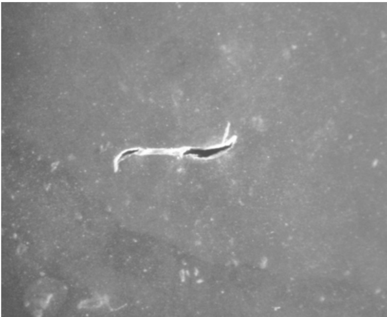
Figure 12.10: Hole caused by a cotton fibre trapped in the rubberfilm.
