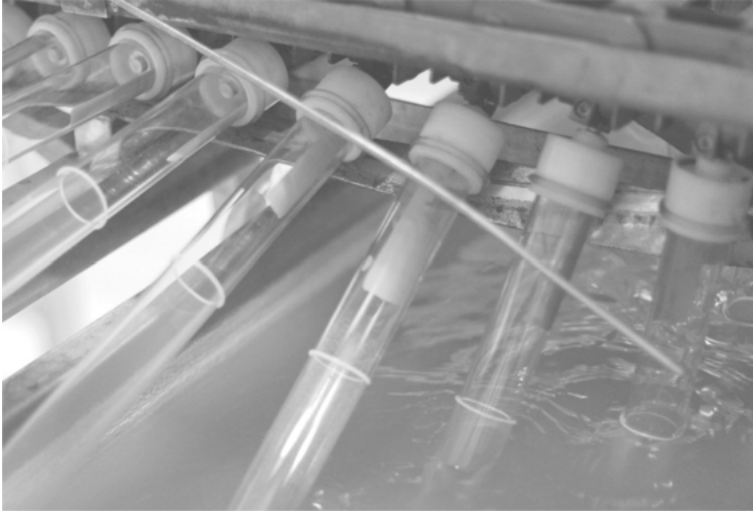
Figure 9.1: Condom formers on a chain plant emerging from the leach tank. Reproduced with permission from the Thai Nippon Rubber Industry Public Company Limited. ©Thai Nippon Rubber Industry Public Company Limited.
