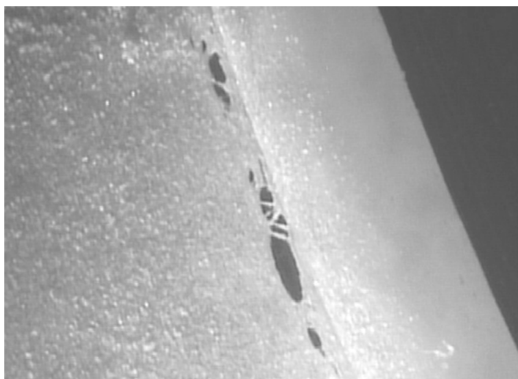
Figure 12.14: Example of holes under the bead of a NR condom.
