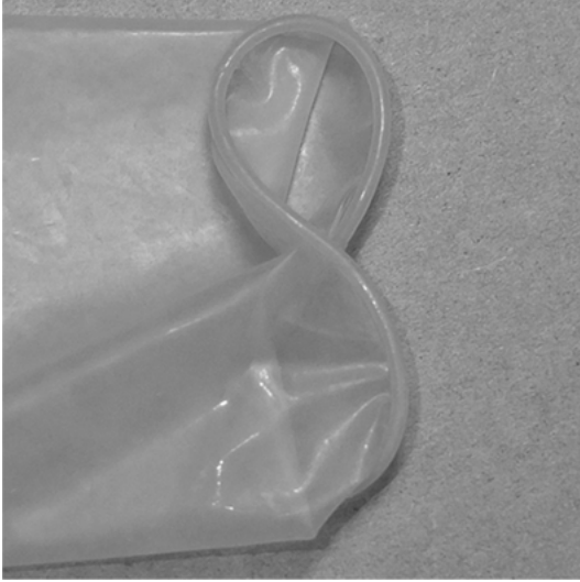
Figure 7.3: A 'figure-8' bead on a condom.
