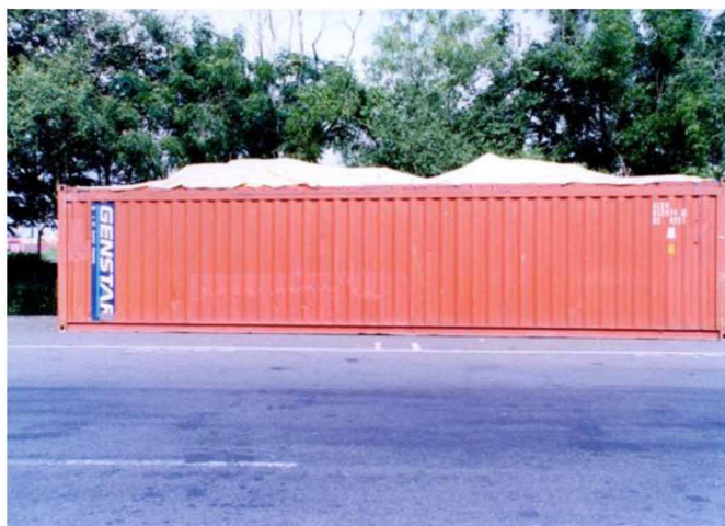
Figure 9. An open top container
