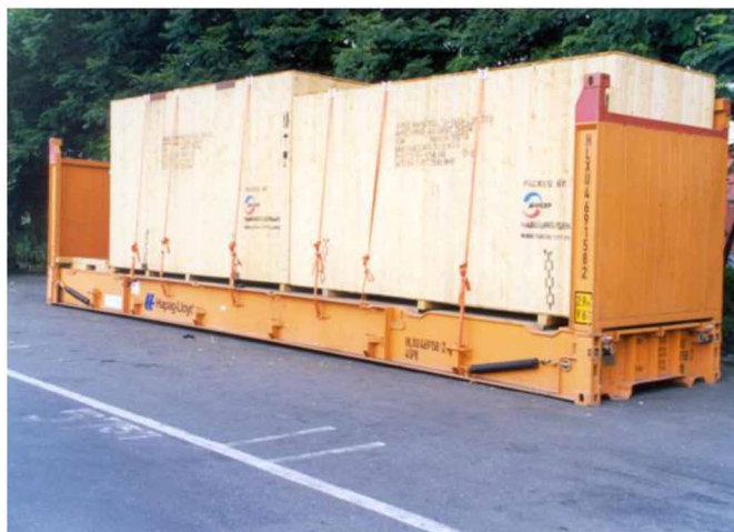
Figure 13. A side and top open container
