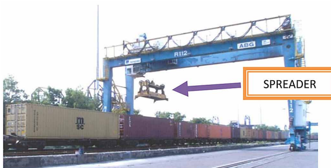
Figure 16. A rail-mounted-gantry crane (RMG)
