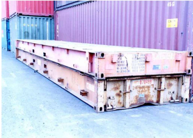
Figure 8. A flat rack container
