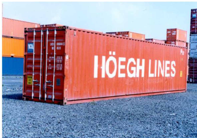
Figure 7. A typical 40' container
