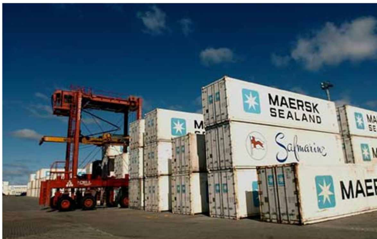
Figure 19. Straddle carrier (SC) stacking containers
