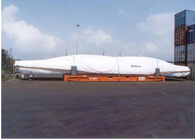
Figure 14. A over dimensioned cargo (out-of-gauge) tied to a flat rack container
