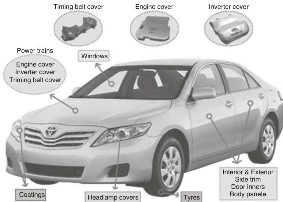
Figure 6.10: The most important parts of a car where polymer nanocomposites are used. Reproduced with permission from Polymer Nanocomposites Drive Opportunities in the Automotive Sector , Nanowerk, 2012. ©2012, Nanowerk [78].
