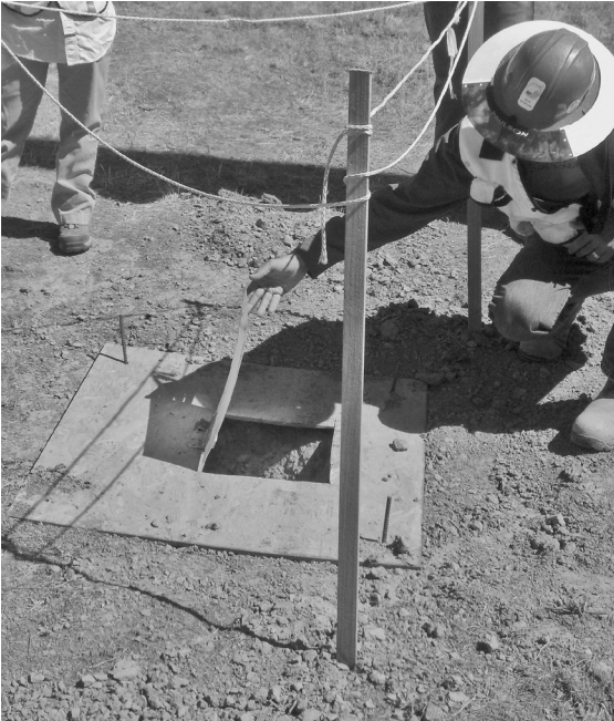
Figure 8.3 Example of a one-way door exclusion device for San Joaquin kit fox. H. T. Harvey & Associates.
