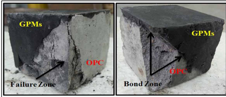
Figure 13. Typical failure model of the GMPs as repair materials
