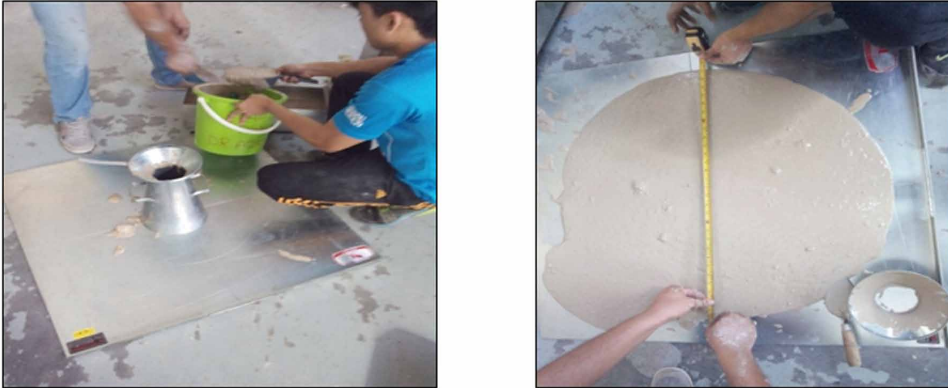
Figure 1. Procedure for slump-flow test
