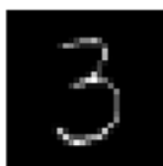
Figure 2.14: Output of the erosion method using OpenCV
