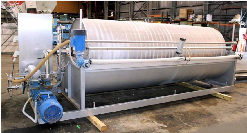
Figure 7. Schematic diagram of Rotary Vacuum Filtration
