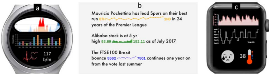
Figure 2. a) Compressed horizon and bar graphs to present fitness activities data, b) Sparklines in texts, c) compressed line graphs to represent heart rate data and sleep quality
