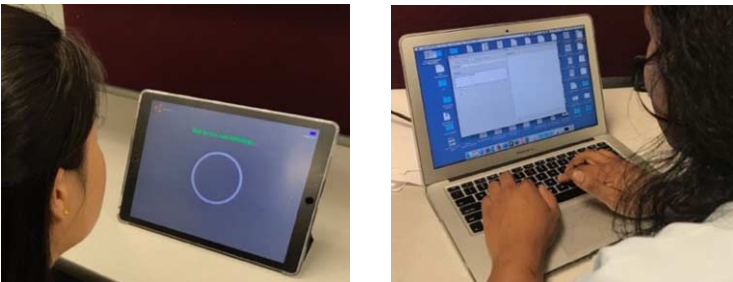
Figure 1. (l) Tablet speech interface using the Siri voice profile, (r) desktop application that provides the tablet's utterances. Both applications were connected peer-to-peer via Bluetooth.
