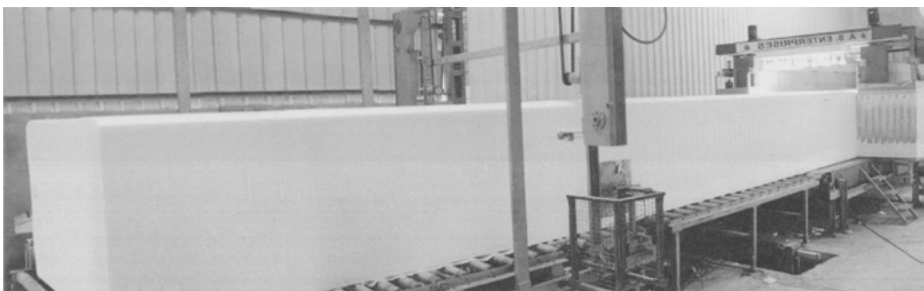
Figure 10.1: PUR continuous F/ Line.
