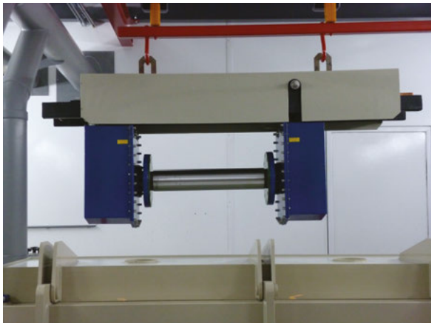
Figure 7.4: Hanging device with rotation motor.
