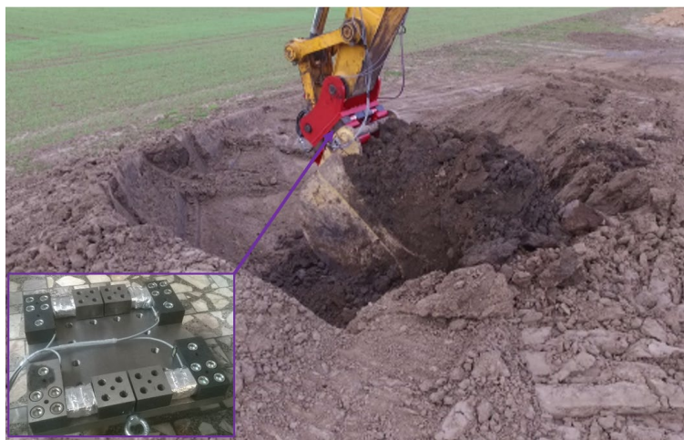
Fig. 8. Measuring beams with protective coatings mounted in the modified quick-coupler during digging
