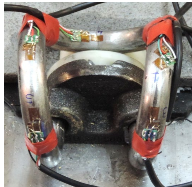
Fig. 6. View of the clip with strain-gauges resistance strain-gauges
