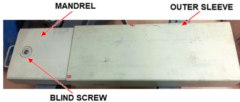
Fig. 2. The main joint of prototype floating bridge
