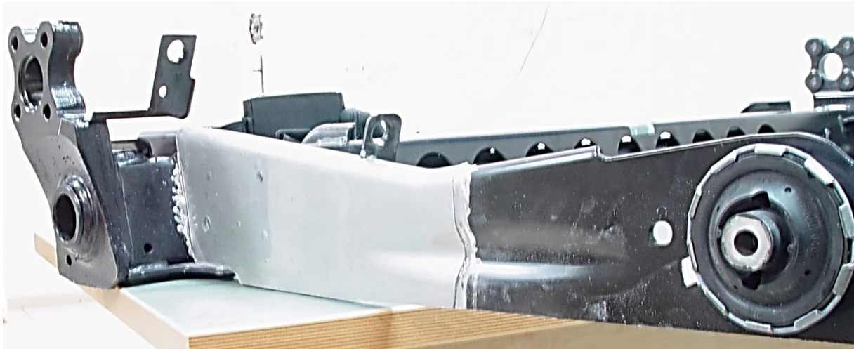
Fig. 1. View of the photoelastic coating on the trailing arm's side surface The rear beam prepared in this way was mounted in the same, technically efficient car model.
