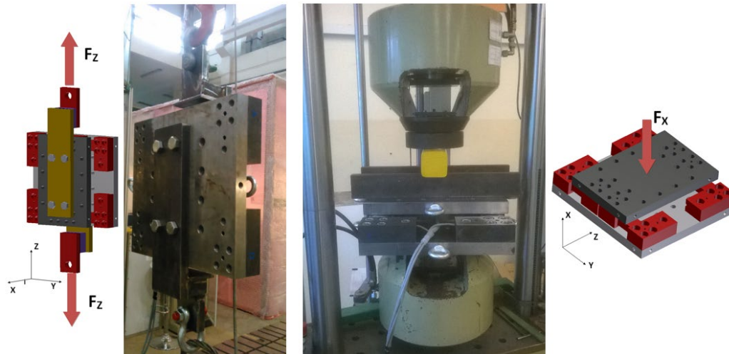
Fig. 5. Laboratory pre-scaling of force and torque sensor loaded with F_z and F_x
