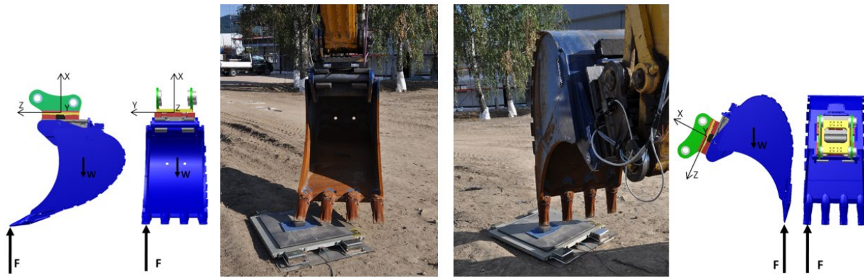
Fig. 7. Final calibration of the sensor prototype allowing the measurement of six load components using bucket and measuring scale
