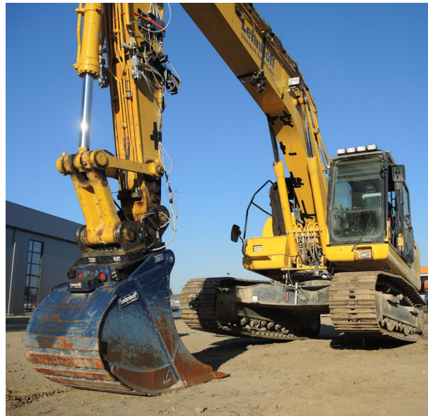
Fig. 6. Komatsu PC210 excavator equipped with modified VL210 quick-coupler with force and torque sensor and bucket during in-situ tests
