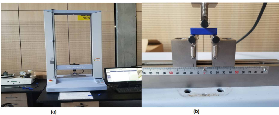
Figure 2. 3 Point bending test a) Machine, b) Specimen during testing
