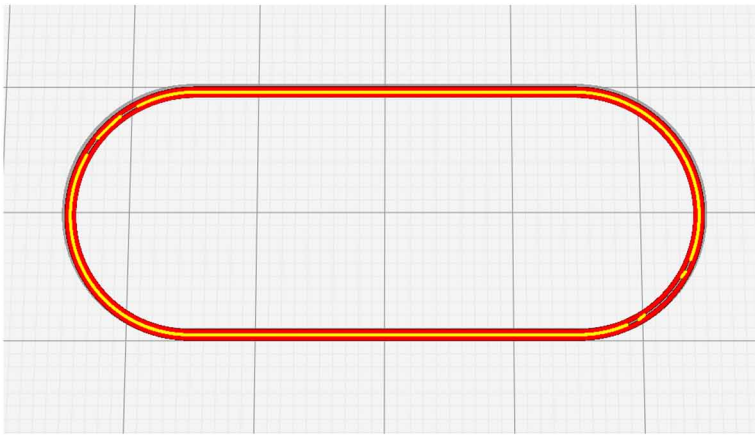
Figure 4. 0.9mm thick test piece simulated with 0.4mm wall thickness showing a solid outer wall and failed infill
