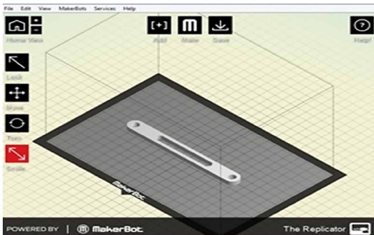
Figure 3. STL file of a 3D part imported into system software of MakerBot
