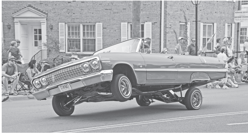
Figure 12.4 1963 Chevy Impala lowrider custom demonstrating hydraulic lift modifications. Photo by Jarek Tuszyński, 2011 (Creative Commons).
