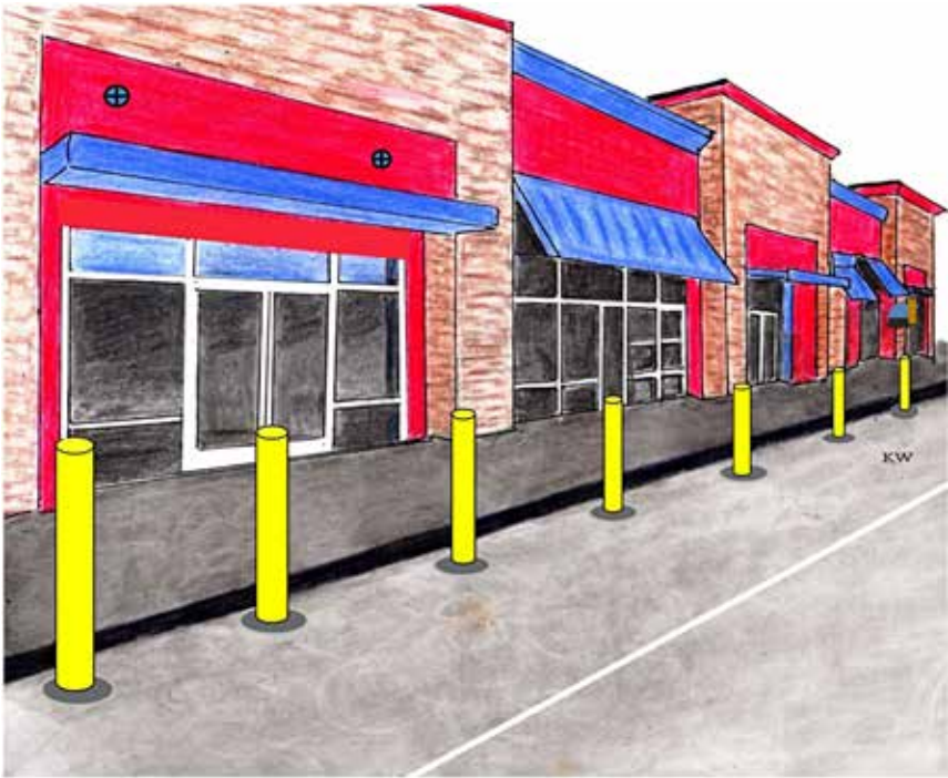
Figure 9.2 Bollard Sequence Placed In Front of Store Fronts and Sidewalks in Order to Protect Store Property and Pedestrians from Rogue and/or Terrorist Drivers. Source: Illustration by F. R. Spellman and Kathern Welsh.
