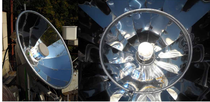
Figure 26. Concentrator solar photovoltaic thermal module, the radiator of which was optimized in the Ansys system of finite element analysis using the developed method
