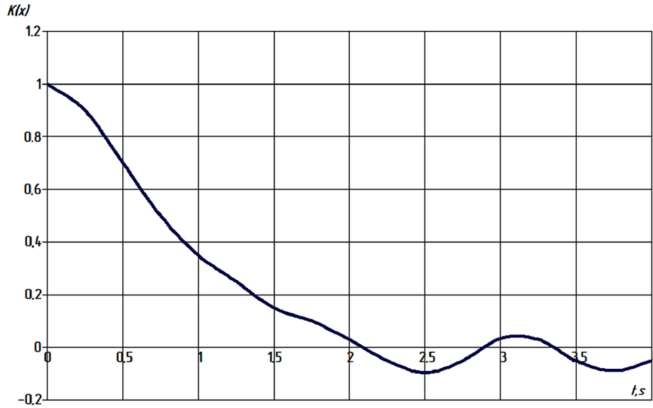
Figure 7. Normalized autocorrelation function effects of the support base microprofile when driving at a speed of 1 m/s
