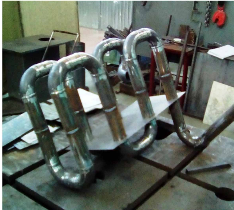
Figure 9. Duct assembly of an experimental vortex recuperative heat exchanger
