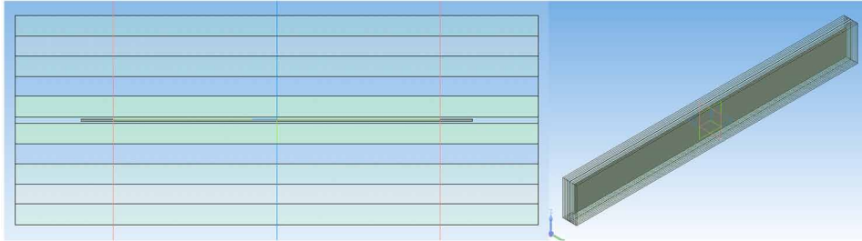
Figure 11. Three-dimensional model of a receiver with a two-sided solar cell and two-sided heat removal (model 4)
