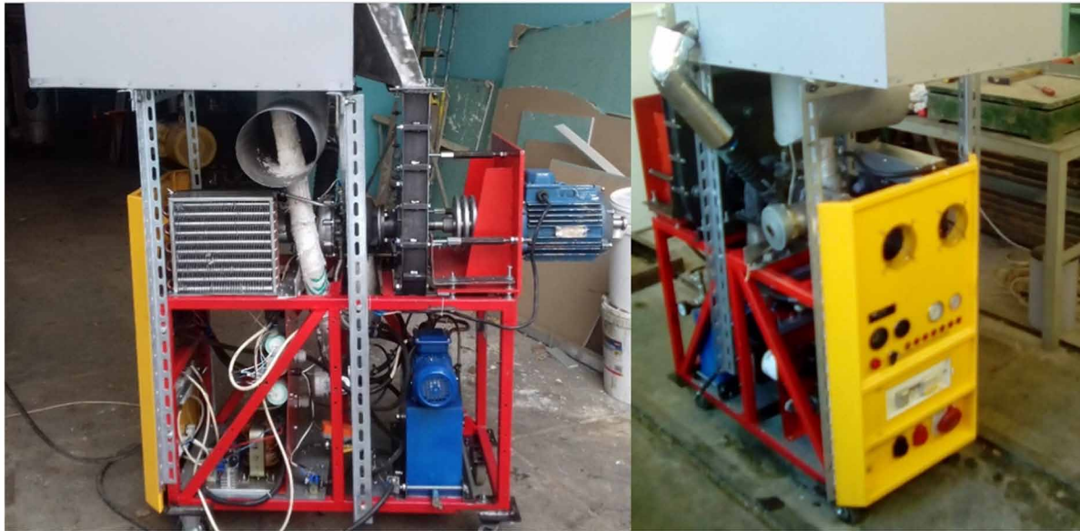
Figure 11. Appearance of a micro gas turbine installation, where a) right side view, b) left side view
