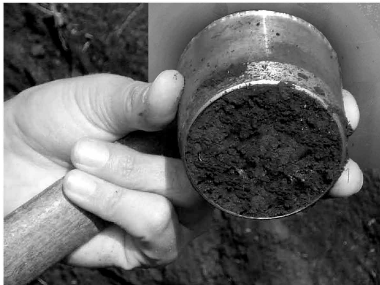
Figure 9. Obtaining a soil sample to determine its density by the method of Kaczynski
