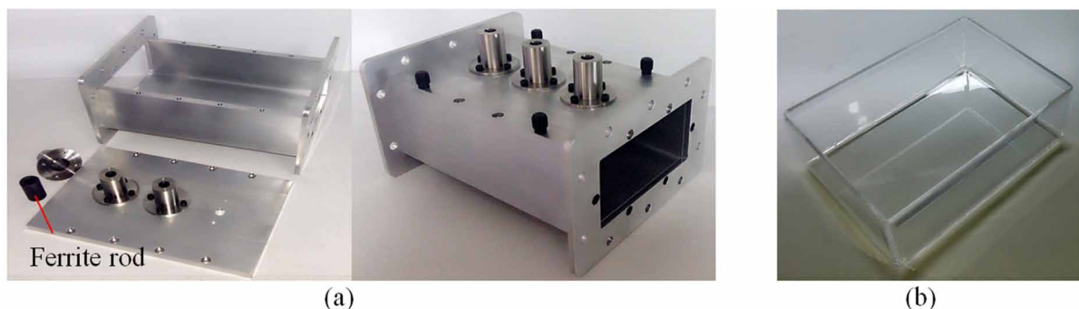
Figure 8. (a) Custom waveguide applicator. (b) Custom quartz glass used as milk specimen holder.
