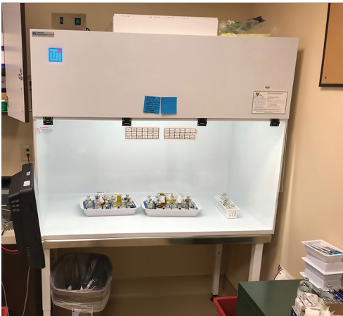
Fig. 16.3 An example of an allergy mixing area with an ISO Class 5, primary engineering control (PEC).
