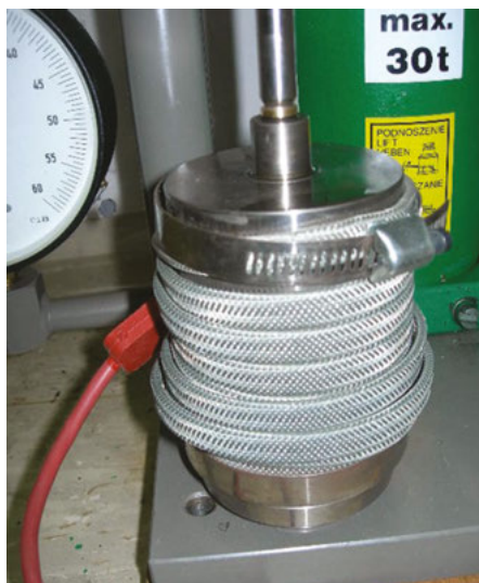
Figure 1.5: External heating of HP reactor chamber.
