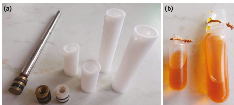
Figure 1.6: PTFE vessels for HP reactions a) PTFE vials and lid extractor tool; b) sealed collapsible PTFE bag.
