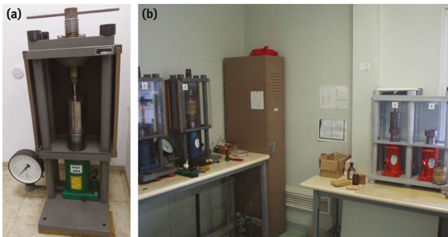
Figure 1.3: HP piston apparatuses (a) at the Ruđer Bošković Institute, Zagreb, and (b) at CQU, Rockhampton.
