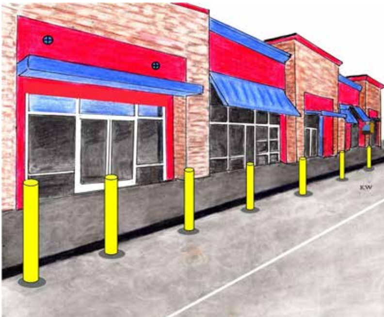
Figure 10.2 Bollard Sequence Placed In Front of Store Fronts and Pedestrian Sidewalks in Order to Protect Store Property and Pedestrians from Rogue Terrorist Drivers using Vehicles of Death and Destruction. Source: Illustration by F. R. Spellman and Katherin Welsh.
