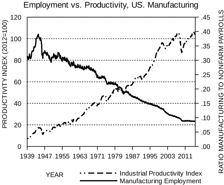
Figure 2.7. Employment vs. productivity, US manufacturing, 1939–2015. Gains in productivity due to automation and mechanization have translated directly into job losses. Data from St. Louis Federal Reserve, INDPRO and MANEMP/PAYNSA data series
