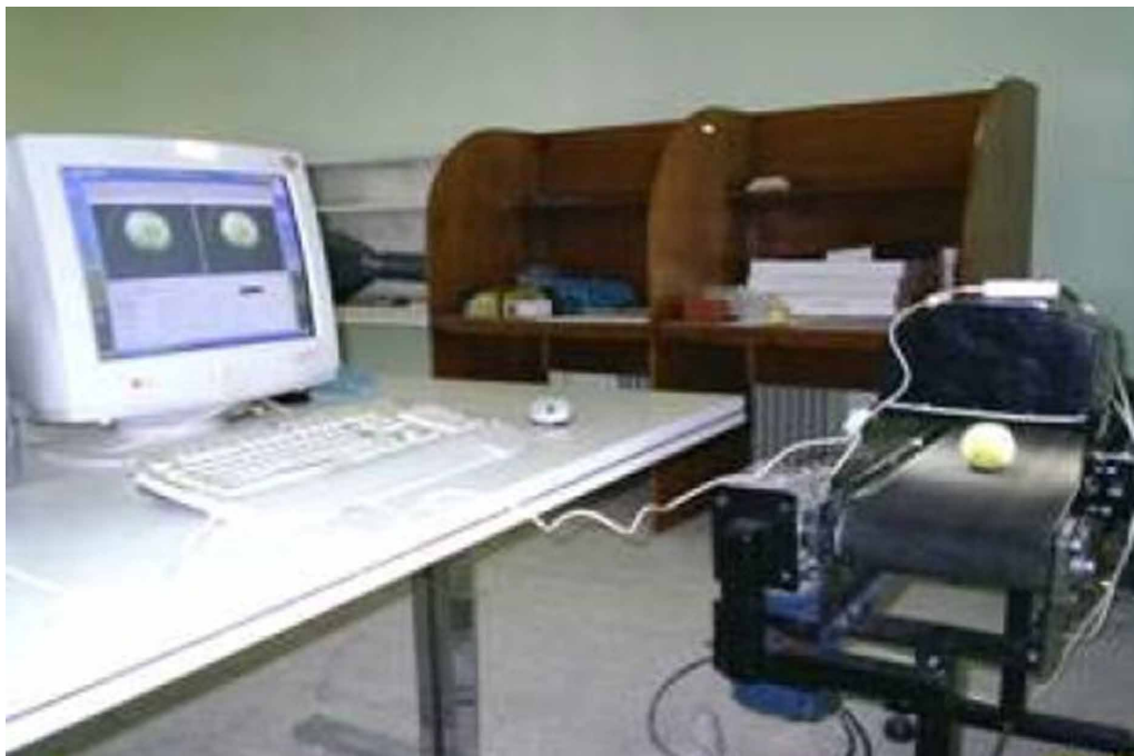
Figure 3. Acquisition system used for apple sorting (Courtesy: Lorestani, A. N. et al., 2006)
