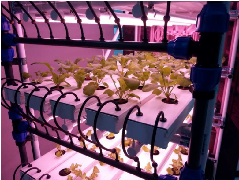
Figure 4: Complex pipework makes more sense for whole season vine crops than short cycle crops.
