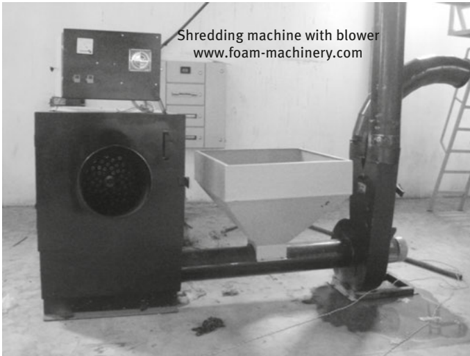
Figure 7.11: Foam waste-shredding machine. Reproduced with permission from Modern Enterprises, India.
