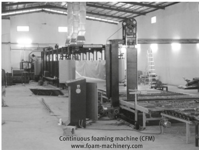
Figure 7.4: Continuous foaming machine. Reproduced with permission from Modern Enterprises, India.
