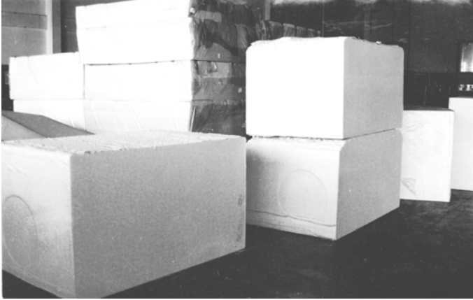
Figure 10.1: Foam blocks after curing and ready for cutting. Courtesy of the author's factory in Sri Lanka.
