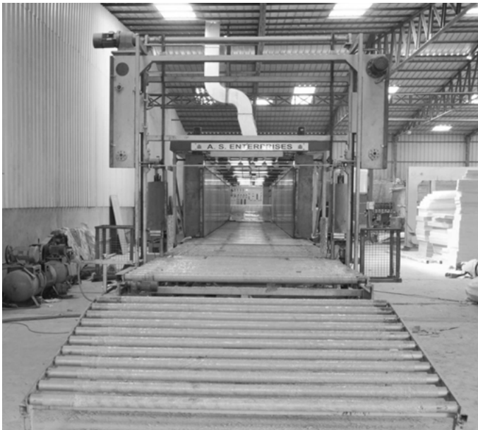
Figure 7.7: Continuous foam-cutting machine. Reproduced with permission from AS Enterprises, India.
