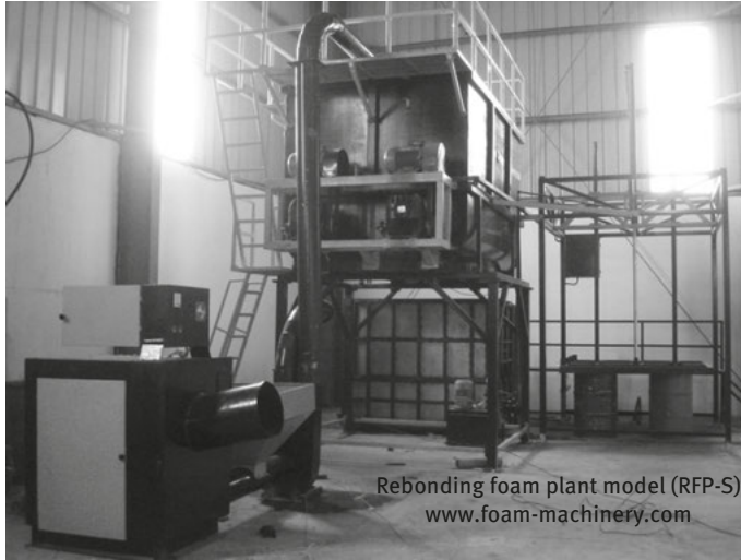
Figure 7.5: Foam waste re-bonding machine. Reproduced with permission from Modern Enterprises, India.
