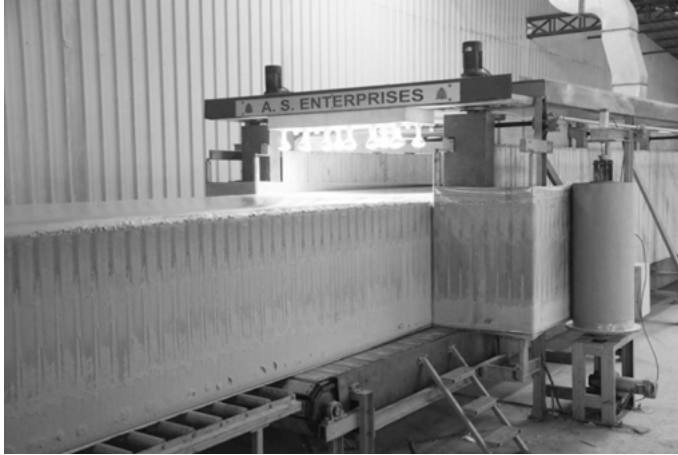
Figure 7.3: Continuous foaming process. Reproduced with permission from AS Enterprises, India.
