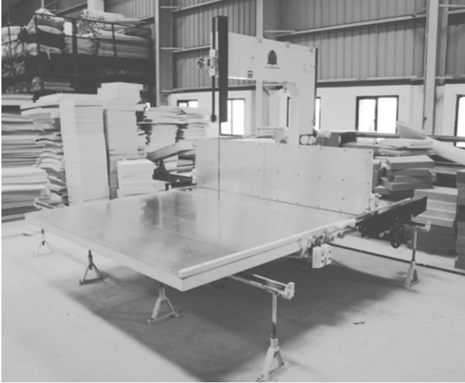
Figure 7.12: Vertical cutting machine. Reproduced with permission from Modern Enterprises, India.
