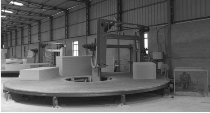
Figure 7.10: Model 3 multiple block-cutting machine. Reproduced with permission from Modern Enterprises, India.
