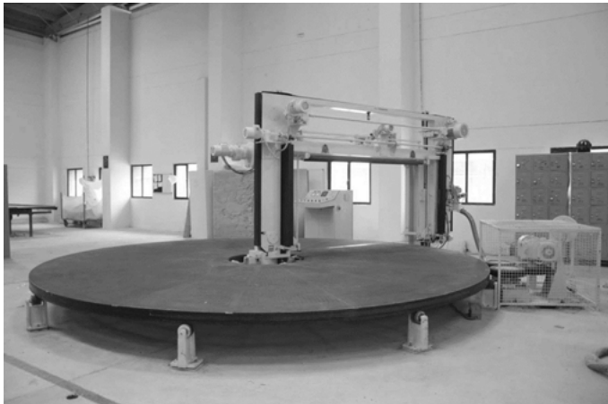
Figure 7.9: Model 2 multiple block-cutting machine. Reproduced with permission from AS Enterprises, India.
