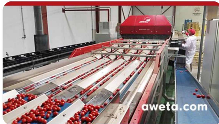
Figure 6. Cherry Tomato Sorter based on Shape, Maturity, Size, and Surface Defects using Machine Vision
