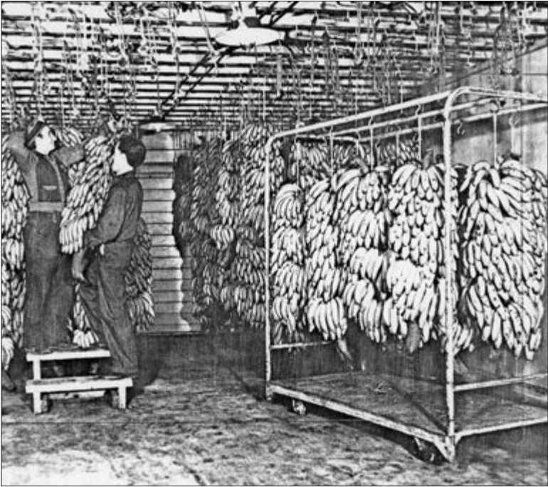
Figure 5.3 A banana ripening room in Springfield, Missouri. The bananas were hung with string and left to rest in the room until the fruit turned to a desirable ripening stage. The roller rack was used for moving bananas between railcar and ripening room (c. 1935). Charles E. Magoon Collection on Produce Marketing, Hagley Museum and Library.
