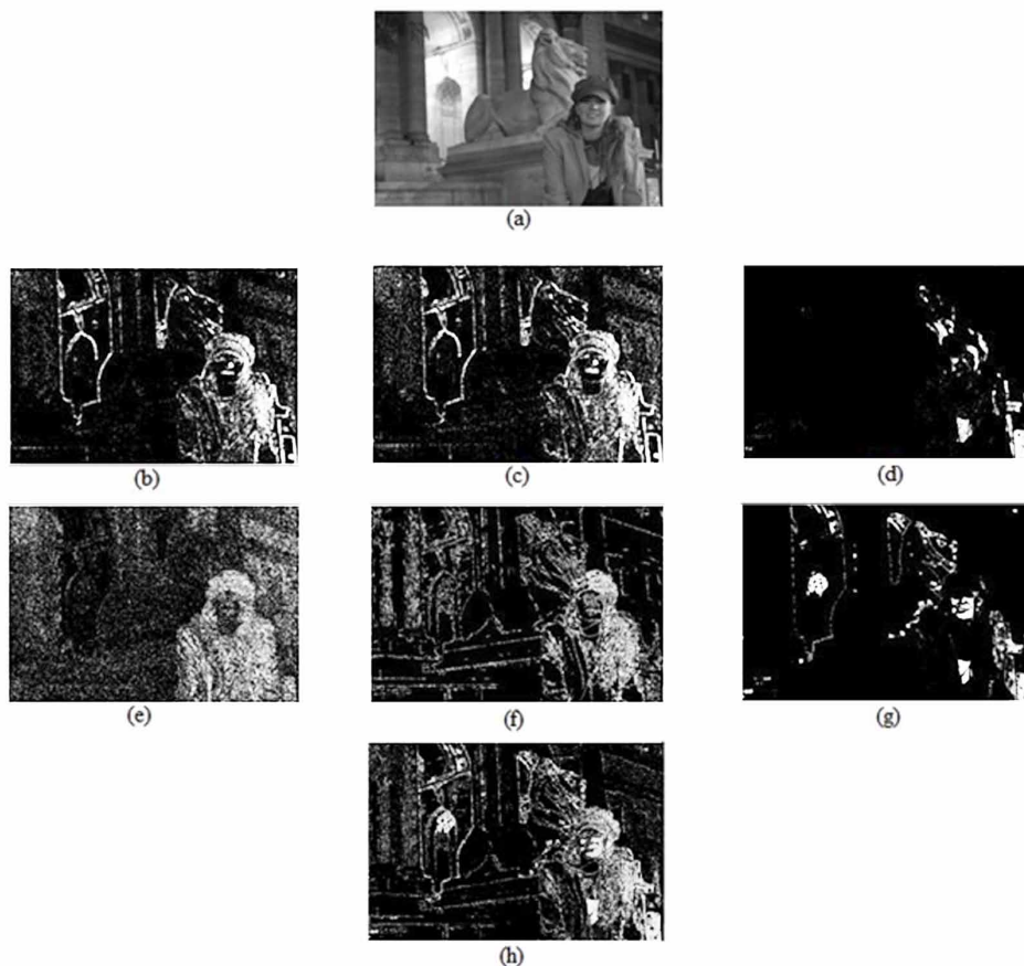
Figure 5. (a) Original mandi image with 3039×2014 pixels. (b) Result by applying Sobel edge detection operator. (c) Result by applying Prewitt edge detection operator. (d) Result by applying Roberts edge detection operator. (e) Result by applying LOG edge detection operator. (f) Result by applying Canny edge detection operator. (g) Result by applying Morphological operator. (h) Result by applying Proposed method.
