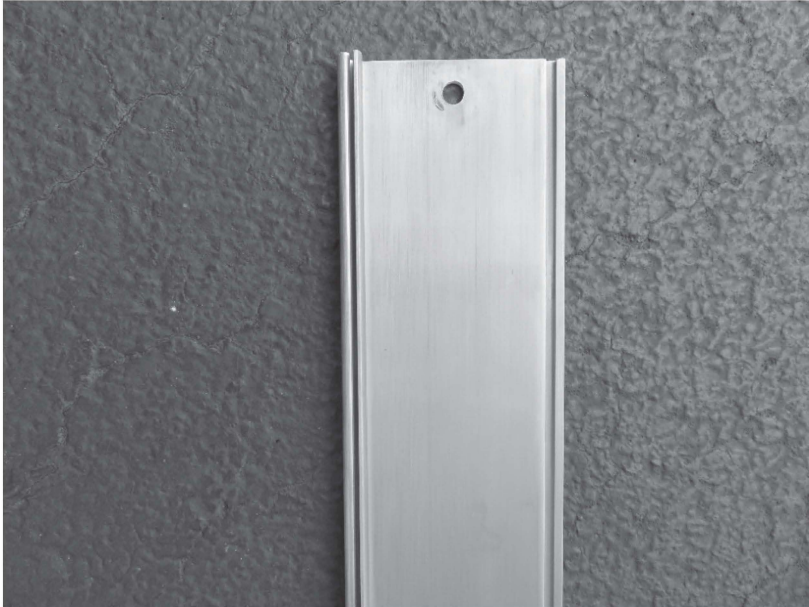
Figure 2.2: Aluminum surface cleaned too strongly and then activated with a strong alkali and conversion coated.
